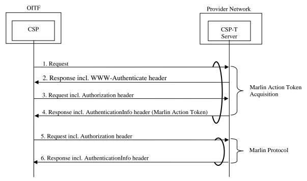
Figure 33: User Authentication for CSP, CSP-T Server communication
