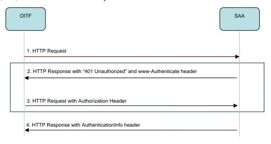
Figure 21: HTTP Basic and Digest Authentication
