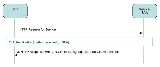
Figure 19: SAA Co-located with Requested Service
