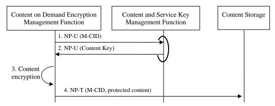
Figure 8: Content on Demand Encryption Sequence using Content Key (for (P)DCF [OMARLIN] or Marlin IPMP [MRL FF])
