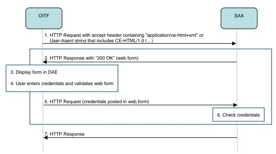
Figure 23: Web Based Authentication with Form
