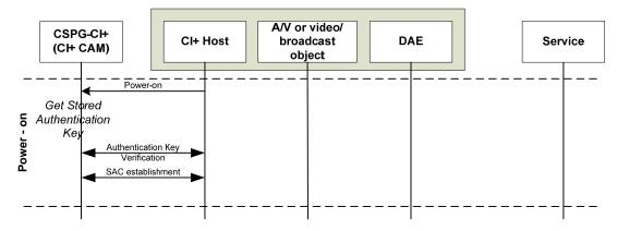
Figure 35: CSPG-CI+ Normal Power-on
