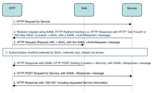
Figure 32: SAML Web-based SSO Authentication
