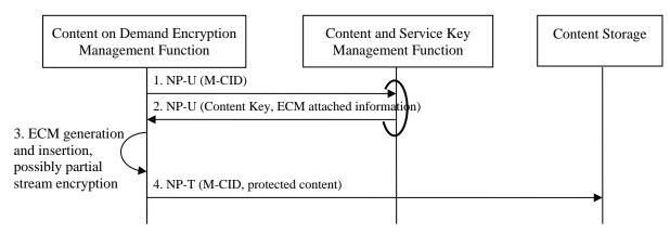
Figure 9: Content on Demand Encryption Sequence using Content Key (for MPEG-2 TS)
