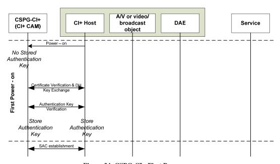
Figure 34: CSPG-CI+ First Power-on
