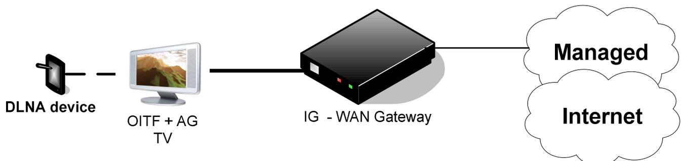
This deployment supports managed and unmanaged services, and DAE and PAE applications. The following devices are deployed:
