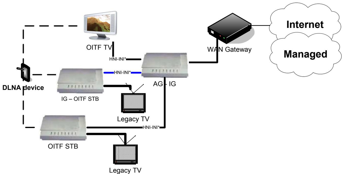
This deployment supports managed and unmanaged services, and DAE and PAE applications. The following devices are deployed:
