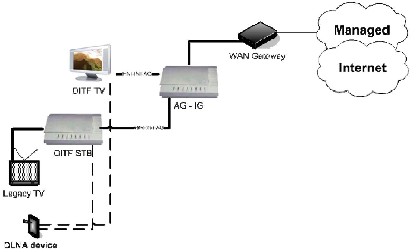
This deployment supports both managed and unmanaged services, with DAE and PAE applications, presented on an OITF TV and a legacy TV. The following devices are deployed:
