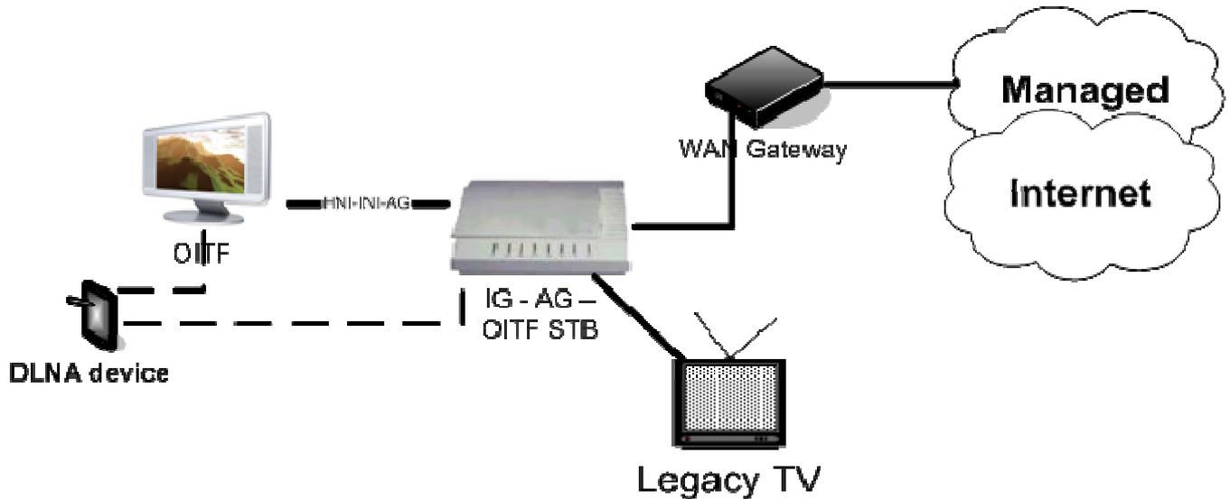
This deployment supports both managed and unmanaged services, with DAE and PAE applications, presented on an OITF TV and a legacy TV. The following devices are deployed:
