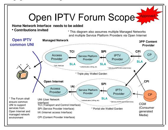
NOTE: In addition to the support of IPTV services delivered via the broadband network the UNI will also support control and information functions for environments where digital broadcast reception (e.g. DVB-S, DVB-C or DVB-T) is integrated in the ITF. This capability is commonly referred to as support of hybrid devices.
