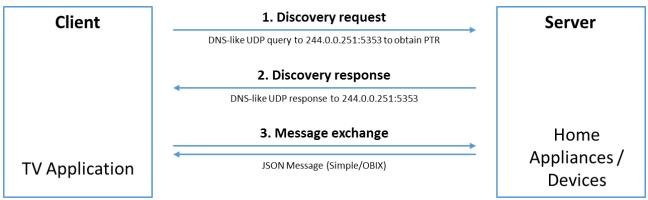
Figure 3 Device Discovery Mechanism using mDNS
